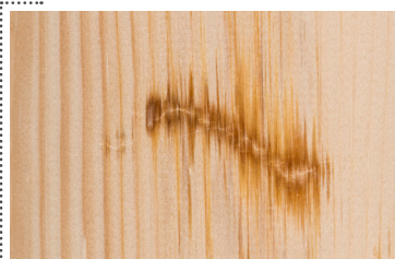
TIMBER BREAK (surrounded by pitch)
