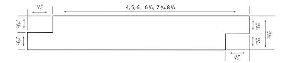
E.W.P. - 6" 8" 10" LOG SIDING NELMA SHIPLAP REVEAL [SIDING]
